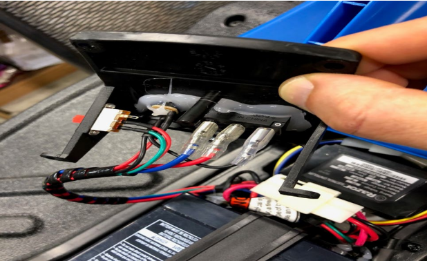
(3) Locate and disconnect all connectors from controller starting from the battery.
