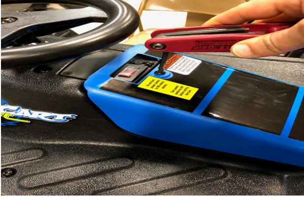
(1) Using a 4mm Allen wrench loosen up the bolt from the plastic cover next to the power switch and lift the battery cover up
