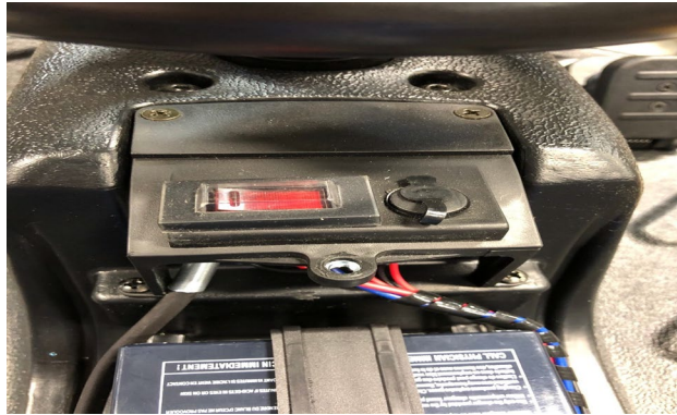
(4) Using a Phillips screw driver remove four screws from the bracket that holds the power switch.
