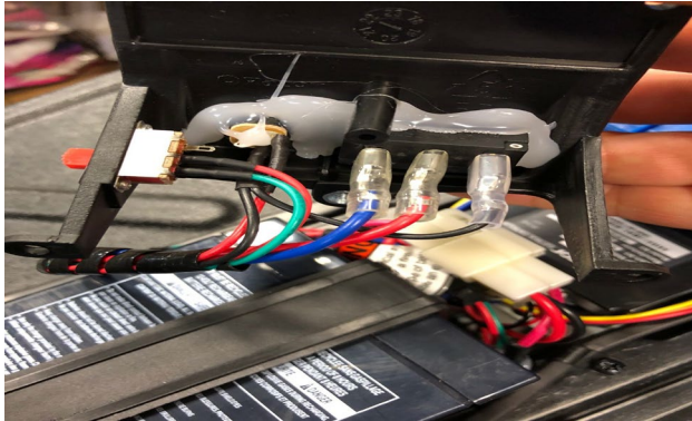
(6) when re-installing the controller always connect the blue wire from controller to the prong closest to the charger port and the red wire to the middle prong.
