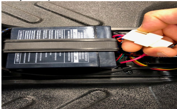
(3) Locate and disconnect all connectors from controller starting from the battery.
