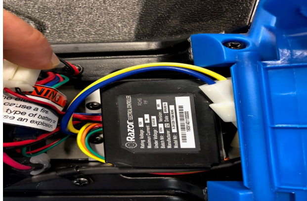
(2) Using a Phillips screw driver remove two screws that hold the controller to the unit.
