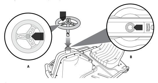
1 Remove the cardboard protector from the steering fork. Insert the steering wheel into the steering fork making sure to align the groove on the steering wheel (A) with the groove on the steering fork (B). Push all the way down.
