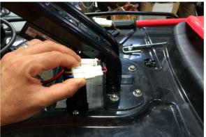
(2) Locate and disconnect motor connector from controller.
