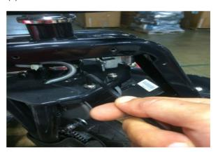
(6) Using a 5mm Allen wrench remove the 4 hex scews that hold the motor to the fork, dismount chain from sprocket and pull motor and cable out from the fork.
