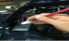
(3) Using a small pointy object from inside the connector depress the locking pins from the prongs and slide prongs out of the connector.
