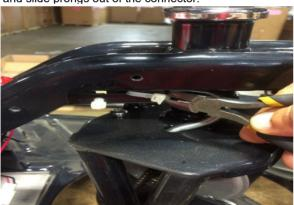
(5) Cut the zip ties that hold the motor cable to the frame.
