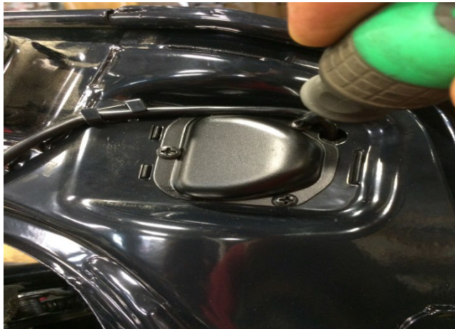
(2) Locate and disconnect the connector from the Throttle to the Controller.
