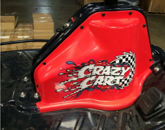
(1) Using a Phillips screw driver remove seven screws from the battery cover from the Throttle side.
