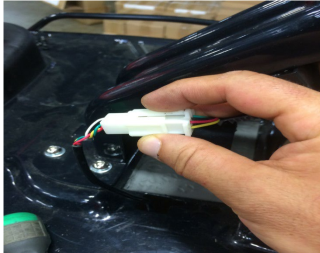
(2) Locate and disconnect the connector from the Throttle to the Controller.
