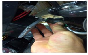
(4) Using a Phillips screw driver remove the screw located on top near the power switch.
