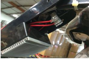
(6) When installing your new Control Module before securing it with the screws make sure to run the two red wires thru the back of the controller and connect them to the two silver prongs on the power switch.
