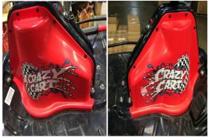
(1) Using a Phillips screw driver remove seven screws from each side of the battery cover and remove both side covers.
