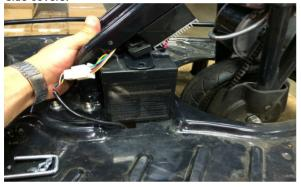
(3) To have better access to the controller remove the battery
