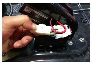
(2) Locate and disconnect all connectors from controller.
