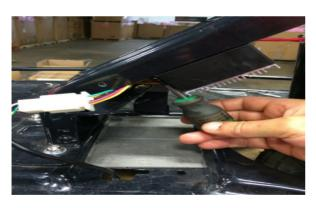
(5) Remove one more screw located at the bottom of controller and remove the controller.
