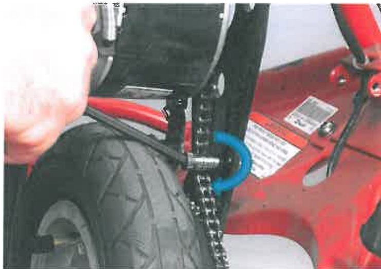
Step 5 – Using a 5mm Allen wrench/Ball driver; carefully align the end of the idler bolt and bearing with the threaded hole on the inner side of the frame then thread bolt through to the other side and tighten with nut. If you do not have a ball driver; deflate the tire to make space to use a 5mm Allen wrench to tighten idler bolt.
