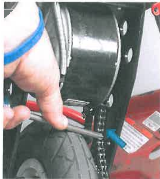
Step 4 - Using a screw driver, carefully push the chain back to expose the threaded hole from the inner side
