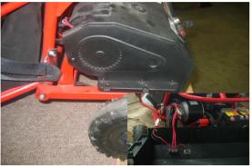
(3) Remove two 4MM hex screws on the left side of the battery cover and 1 phillip screw located in the middle left side of the battery cover and remove the cover away from the unit carefully not to pull the wires connected to the power switch or charger port.
