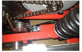
(5) Dismount the chain from the axle sprocket, by releasing the tension from the chain tensioner and carefully turn the axle as you push the chain out of the sprocket.
