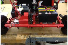
(6) Using a 6mm Allen wrench remove two bolts from each side from the bearing holder and remove the axle, remove wheels from axle and replace the disc brake.
