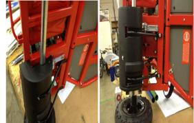
(4) Flip the unit on the side to get acces to the bottom part of the motor cover, Using a Phillips screw driver remove the screw located on the side ands using a 5MM Allen wrench remove the 3 hex bolts that hold it onto the frame and remove.
