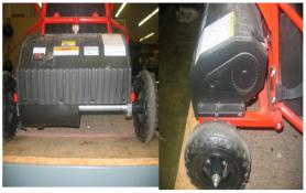
(1) Using a 17mm open wrench loosen up the nut located at the center of the rim, wrench must turn counter clock wise to loosen up the nut, you can apply the brake of the unit to prevent the wheel from turning as you try to loosen up the nut.
