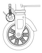
**3** If the brake is too tight or too loose, use a 8 mm wrench and a 3 mm Allen wrench to adjust as needed.
