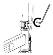
**2** With the front wheel pointed straight ahead, the handlebars square to the front wheel and the Razor logo facing the front, use a 5 mm Allen wrench to tighten the two (2) bolts on the collar clamp. The collar clamp is properly tightened when the handlebars cannot be twisted out of alignment with the front wheel.
