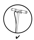
**Note:** The cable assembly from the handlebar must not wrap around the handlebar stem. Sharp bends or twisting of the brake cable can cause the brake to malfunction.
