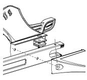
**2** Align the holes on the right and left platforms with the holes on the frame.
