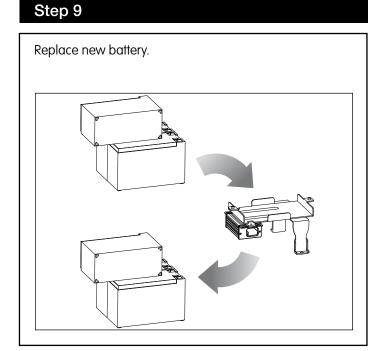
Put the battery bracket (lower) and battery back onto the frame.
