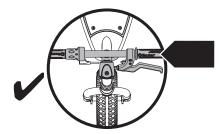
WARNING: Failure to properly tighten the collar clamp may allow the handlebars to dislodge while riding and may cause you to lose control and fall. When correctly tightened, the handlebars will not rotate out of alignment with the front wheel under normal circumstances.
