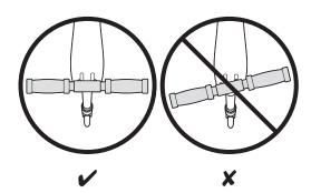
**3** Point the front wheel straight ahead, square the handlebars to the front wheel and face the Razor logo to the front.
