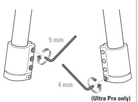
**4** Tighten the clamp as shown. Alternately tighten each bolt until the clamp is tightened securely.
