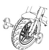
**3** Slide axle bolt through the front fork, spacer and wheel hub. When axle bolt passes through the other side of the wheel hub, add the other spacer, and slide through the front fork. Secure with washer and nut.
