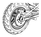
**1** Loosen the two (2) Phillips screws and remove chain guard.
