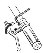
**3** Adjust the brake levers to the proper place and tighten it with the 5 mm Allen wrench.
