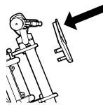
Align the two (2) tabs on the plate with the holes on the front fork and carefully push inward until plate clicks securely into place.
