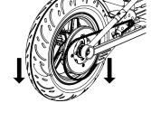
**3** Push the chain tensioner down to loosen the chain and remove the chain from the wheel sprocket and motor sprocket. Push wheel downward to remove.
