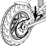
**4** Install the new chain or wheel by slipping the chain around the axle bolt. Slide the axle bolt into the slots on the frame. Slide the chain tensioner down and maneuver the chain onto the rear sprocket and motor sprocket.
