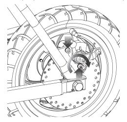
**AWARNING:** Failing to properly adjust and tighten the nuts and bolts that affix the rear wheel can cause you to lose control and fall.
