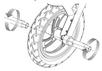
**AWARNING:** Failing to properly adjust and tighten the nuts and bolts that affix the front wheel can cause you to lose control and fall.
