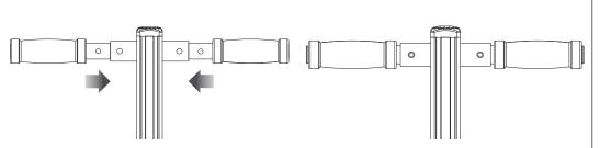
**1** Insert and secure the left and right handlebars by pressing the spring-loaded buttons and inserting them into the main shaft.
