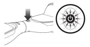
**2** Turn power **ON.** If product remains level or adjusts to become level, calibration has been confirmed. No further steps are needed.
