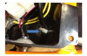
5) Carefully slide the brake connector through the opening located at the back of the battery tray and remove brake assembly.
