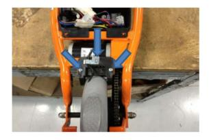
2) Remove the (2) two Phillip screws on battery strap and carefully remove battery from battery tray.
