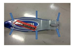
1) Using a Phillips screwdriver, remove the (6) six screws on the deckplate
