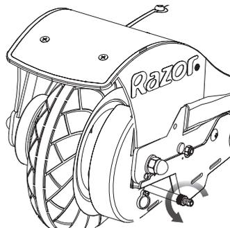
**2** Open the round cover located on the chain guard by sliding the cover downward. Align the opening in the sprocket with the valve stem. Thread the valve extender completely onto the valve stem and attach the pump. Inflate to the PSI indicated on the tire sidewall.
