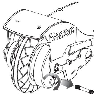
**3** Remove valve extender immediately after inflating and close the round cover.
