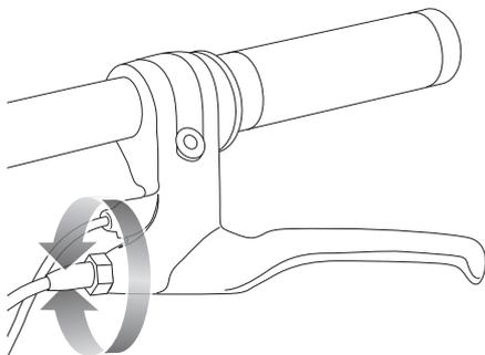
**1** To adjust the brake cable tension, thread the brake lever adjuster in or out 1/4 to 1/2 turn until the desired brake adjustment is attained. Most adjustments are complete at this step. If brake still needs further adjustment, proceed to step 2.
