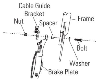
**7** Install the cable guide bracket to the frame and brake plate using bolt, washers, and nut. Do not tighten.
