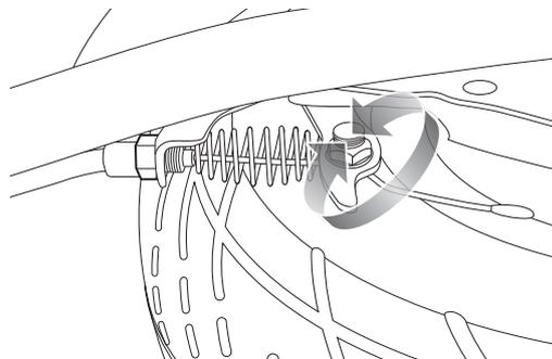
**2** If the brake is too tight or too loose, use a 10 mm wrench to loosen the nut for additional adjustment on the brake cable. Securely tighten the nut when finished.
