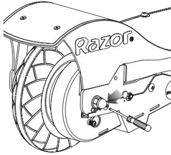
**1** With a Phillips screwdriver, loosen the three (3) screws on the chain guard and remove.
