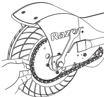
**5** Install the chain onto the rear wheel sprocket. Slip wheel axle into the frame slots. See rear wheel hardware sequence on prior page. Push the chain tensioner down to create slack in chain. Hand tighten rear axle locknuts.
