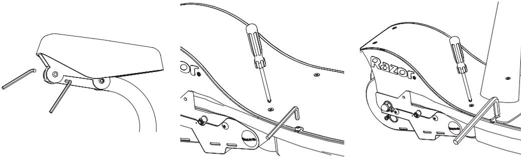
**1** Attach the seat to the seat post with two (2) 4 mm Allen wrenches. See note below.
