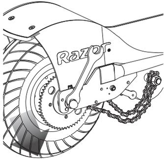
**4** With two (2) 16 mm wrenches, loosen the axle locknuts. Push down and remove wheel from the frame. Remove chain from rear sprocket.
