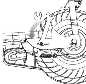
**3** With two (2) 8 mm wrenches, remove the cable guide bracket from the frame and brake plate. Keep the bolt, washer, spacer, and nuts together.
