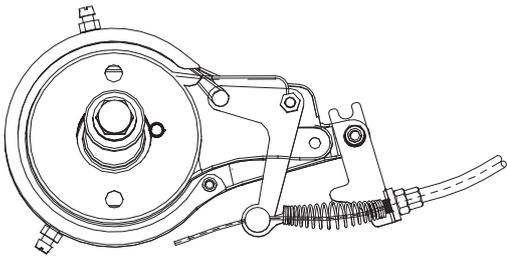
**8** Thread the brake cable through the brake adjuster barrel, through the large spring, and into the small hole in the side of the anchor bolt. Position the cable to the original location (as indicated by the slight cable kink) and tighten securely.
