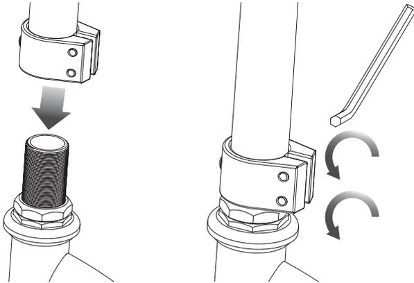
**1** Loosen the collar clamp. With a twisting motion, push and twist to slide the handlebar onto the fork.
