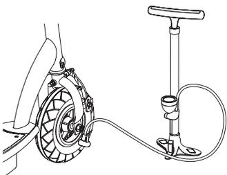
**4** Using a bicycle style tire pump equipped for a Schrader-type valve, inflate the front tire to the PSI indicated on the sidewall of the tire.
