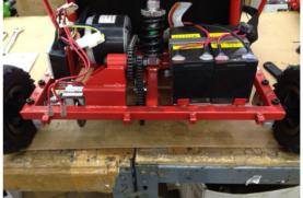
(6) Using a 6mm Allen wrench remove two bolts from each side from the bearing holder and remove the axle, remove wheels from axle and replace the disc brake.
