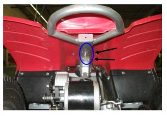
4) Using a size 10mm wrench, remove two lock nuts underneath the rear fender
