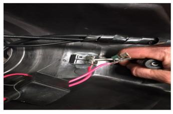
7) Remove the plastic cover from the back of the power switch and using a flat screw driver remove the wires and silicone from around the power switch.
