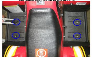
3) Using a 5mm Allen wrench, remove the 4 bolts on both sides of the footrest platforms
