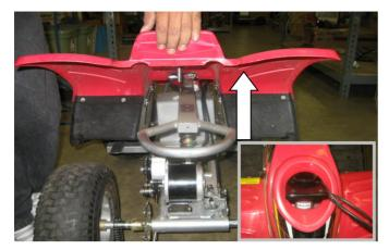
5) Lift up the plastic body. Carefully maneuver the front of the body plastic around the top of the steering tube (See insert)
