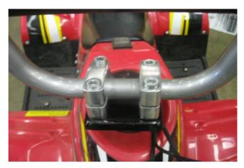
2) Using a 6mm Allen wrench, remove the 4 bolts on the handlebar clamps and detach handlebars
