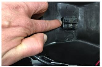
8) De-press the locking tabs from the power switch and push out switch from body fairing.
