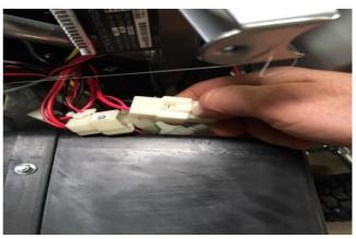
6) Disconnect the wire harness from the power switch to the controller and batteries also disconnect the charger port connector from controller.
