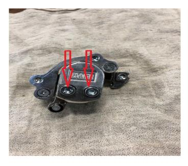
(1) Using a 5mm Allen wrench remove the two hex bolts shown on the picture
