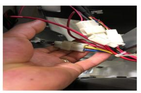
(2) Locate and desconnect the motor from controller.
