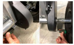
(4) Using a Phillips screw driver remove two screws located on the bottom inner side of the chain guard, remove one more screw to allow the chain gurd to be split in half.
