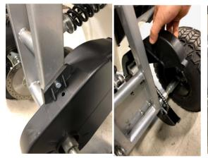
(5) Using a 5mm Allen wrench loosen up and remove the hex bolt that holds the chain guard to the frame, split the chain guard in half and remove.
