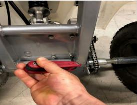
(6) Using a 5mm Allen wrench loosen up and remove 4 hex bolts that secure the motor to the frame, tilt the motor to the side and remove the chain off from the motor sprocket.
