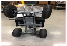
(1) Being very careful lift and rest the unit on the back wheels.
