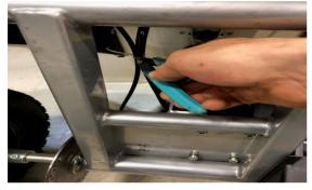
(3) Cut the zip tie that holds the motor wire to the brake cable.
