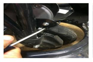
(3) Remove 3 screw located on the chain guard and remove the chain guard.
