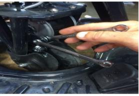
(4) Using two 10MM wrenches loosen up the luck nut that secures the tensioner on to the fork and remove it.
