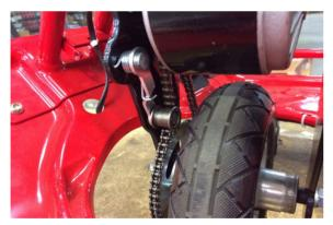
(5) Chain tensioner roller should always be on the outter side of the chain putting pressure against the chain.
