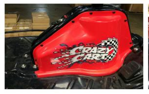
(1) To have better access to the chain tesioner, Using a Phillips screw driver remove 7 screws from the motor cover.
