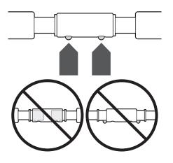
**4** Make certain **BOTH** handlebars are properly locked onto the T-bar.
