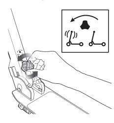
**1** To fold scooter you must first deactivate the Anti-Rattle feature. Turn the knob counterclockwise to loosen.
