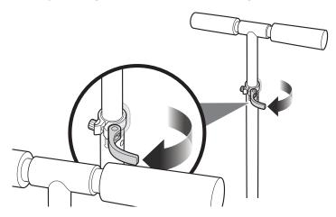
**1** To adjust the height of the handlebars, open the quick-release lever and slide the T-bar to the desired position and resecure the quick-release lever to lock into place.
