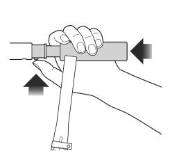
**3** Insert and secure the left and right handlebars by pressing the spring-loaded buttons and inserting them into the T-bar.
