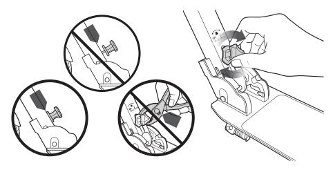
Note: To activate the Anti-Rattle feature, turn the knob clockwise. Note there is no need to overtighten.
