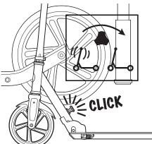
**2** Turn knob clockwise to tighten and engage the Anti-Rattle mechanism.
