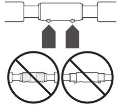
**4** Make certain **BOTH** handlebars are properly locked onto the T-bar.
