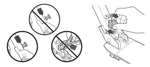
Note: To activate the Anti-Rattle feature, turn the knob clockwise. Note there is no need to overtighten.
