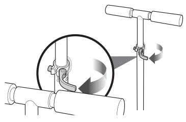
**1** To adjust the height of the handlebars, open the quick-release lever and slide the T-bar to the desired position and resecure the quick-release lever to lock into place. **Note:** When the T-bar is raised to the maximum height, depress the push button located directly below the quick-release lever to unlock the T-bar.
