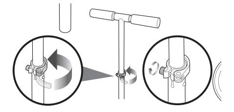
**2** The tension of the quick-release lever can be adjusted by manually tightening or loosening the Allen bolt. Be careful not to over-tighten. You should always be able to open and close the quick-release lever by hand and the T-bar should slide freely when the quick-release lever is open.
