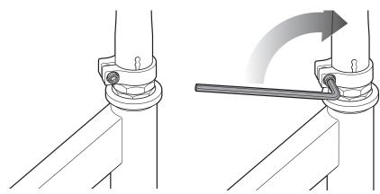
Using a 5 mm Allen wrench, check that the collar clamp bolt is tightened securely. This item is tightened and quality inspected at the factory, but there is a slight chance that the effects of shipping or handling may have caused the bolt to loosen.
