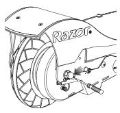
**1** With a Phillips screwdriver, loosen the three (3) screws on the chain guard and remove.
