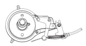
8 Thread the brake cable through the brake adjuster barrel, through the large spring, and into the small hole in the side of the anchor bolt. Position the cable to the original location (as indicated by the slight cable kink) and tighten securely.
