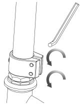
**2** With the front wheel pointed straight ahead and the handlebars square to the front wheel, tighten both bolts on the clamp as shown with a 5 mm Allen wrench. Tighten securely.
