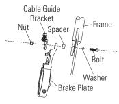
7 Install the cable guide bracket to the frame and brake plate using bolt, washers, and nut. Do not tighten.
