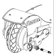
**3** Remove valve extender immediately after inflating and close the round cover.
