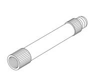
**1** Use the included valve extender located in the end of the right handlebar grip.
