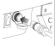
**2** Make sure the power is in the **OFF** position. Plug the charger into the charger port on the product. The light on the charger should turn red during charging. The light will turn green again when charging is complete.
