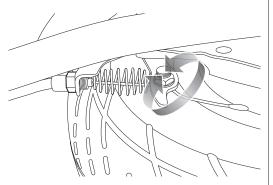
**2** If the brake is too tight or too loose, use a 10 mm wrench to loosen the nut for additional adjustment on the brake cable. Securely tighten the nut when finished.
