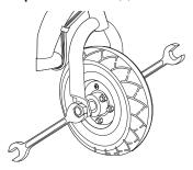
1 Using two (2) 16 mm wrenches, loosen the front axle bolts by turning the wrenches counter clockwise. Remove wheel and install replacement wheel. Note the sequence of the hardware.
