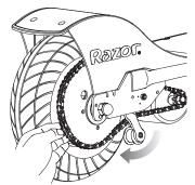
**6** Verify chain is properly installed on each sprocket and tensioner is correctly positioned at the bottom of the chain.
