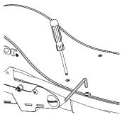
**2** Remove the four (4) screws on the middle of the deck with the 4 mm Allen wrench and the Phillips screwdriver.
