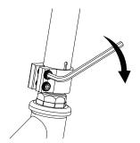
**2** With the front wheel pointed straight ahead, the handlebars square to the front wheel and the Razor Logo facing the front, tighten the clamp as shown. Tighten securely.
