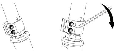
Using a 5mm allen wrench, check that the collar clamp bolt is tightened securely.
