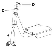
**1** Remove the black protective cover from the top of the fork. Slide the collar clamp (D) up the fork and remove. Remove washer (C) from fork. Insert the front fork into the steering tube. Slide washer (C) back onto the front fork. Slide collar clamp (D) back down onto the fork until it is sitting directly on top of washer (C).
