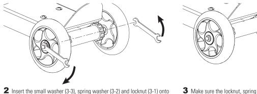
Insert the small washer (3-3), spring washer (3-2) and locknut (3-1) onto the axle bolt and tighten securely using (2) 10mm wrenches.
