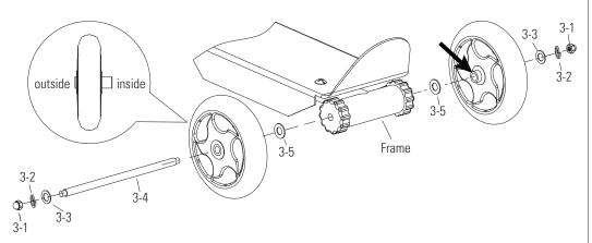
**1** Remove the locknut, spring washer and washers (x3) **from one side** of the axle bolt. Insert the axle bolt through the rear wheel making sure the long spacer on the wheel (refer to arrow above) is facing towards the frame. Insert the large washer (3-5) onto the axle bolt between the frame and rear wheel and slide the axle bolt through the frame. Slide the other large washer and wheel (with the long spacer facing inwards towards the frame) onto the axle bolt.
